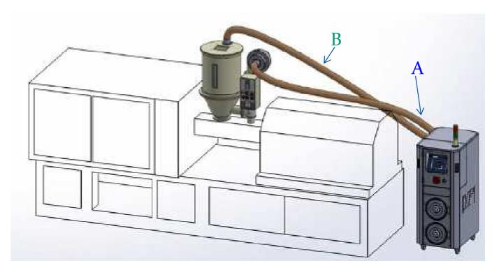
A: YP乾燥机送乾燥的风送至料桶中 A: YP dryer send drying wind into hopper.
